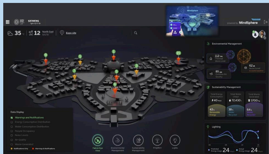
A dashboard showing the ‘digital twin’ of the Expo 2020 (and soon to be District 2020) site whereby the industrial internet-of-things platform collects data from sensors located across the site to maintain every aspect of the operation e.g., energy, water supply, electricity, traffic, and incidents. Photo credit: Siemens
